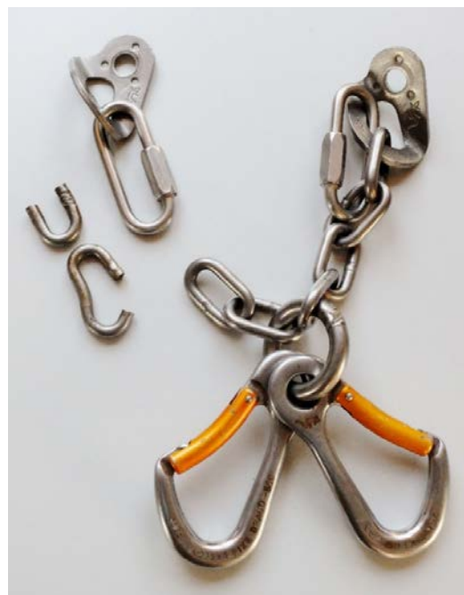
Photo 1: FIXE belay anchor with two broken chain links.
