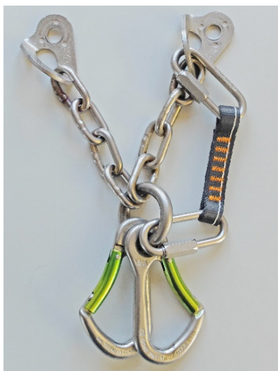
Photo 2: example of a temporary backup for the chain.
