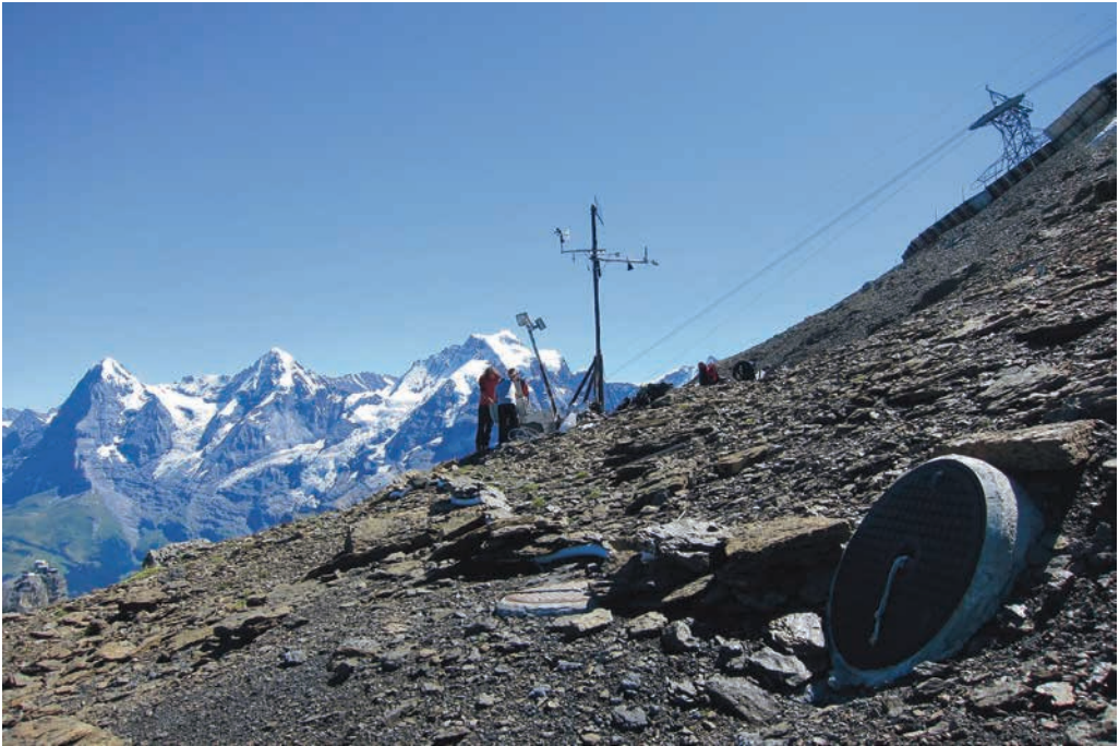
Figure 3.7: Borehole site at the Schilthorn, Bernese Oberland. The covers for borehole SCH_5200 (right) and SCH_5000 (centre, flat) can be seen in the foreground, the energy balance and borehole measurement station and the smaller mast of the automatic ERT are seen in the back. The borehole station was renovated in summer 2011. Photo: J. Nötzli, August 2011.
