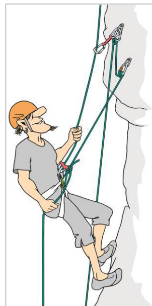
Figure 2: Belaying off the harness is more comfortable – but only possible if the space above the belayer is free from obstacles and when a sufficiently long self-belaying sling and dummy runner or plus-clip is used.
