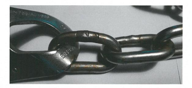
From the International Mountaineering and Climbing Federation (UIAA) of which we are members, also they inform us that have been detected in different countries some faulty anchors from different manufacturers by problems of corrosion cracking under stress, also known as Stress Corrosion Cracking (SCC)
