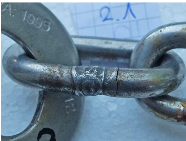
Figure 2: Chain link showing average traces of corrosion and an obvious fissure.
