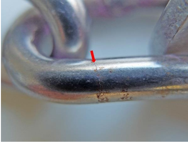
Figure 3: Chain link showing a fine fissure opposite to the weld seam.
